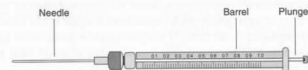
Figure 2-13 Hamilton syringe with a volume of 1 \mu\text{L} and divisions of 0.02 \mu\text{L} on the glass barrel. [Courtesy Hamilton Co., Reno, NV.]
